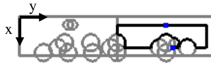
Figure 67. Contact point 1 pin location for span 4 inches to 8 inches
